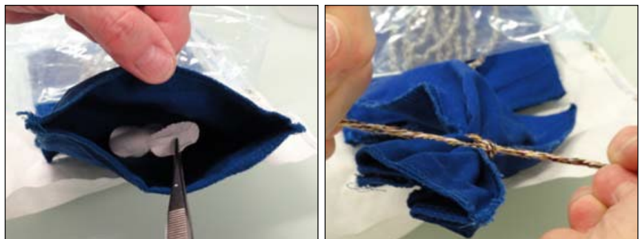
Fig. 1: Per test germ, 5 biomonitors are transferred into a blue cotton bag. The cotton bag is sealed.
