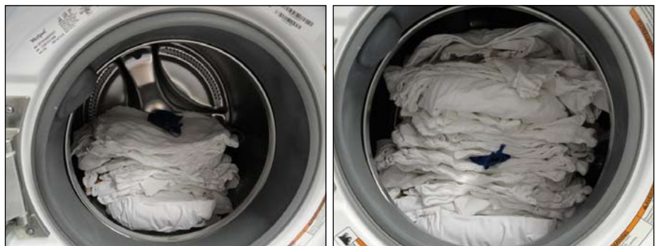
Fig. 2: The cotton bags are placed in the middle of the load without touching each other
